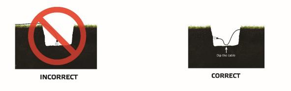
Figure 2.7 Horizontal placement sensor and dipping the cable is recommended
