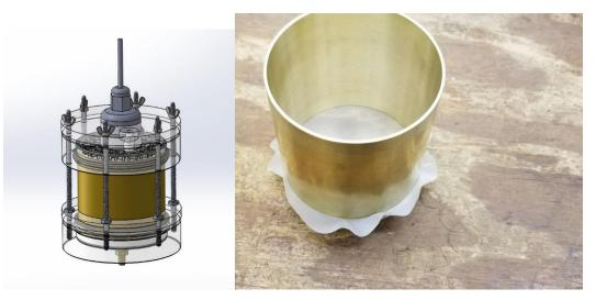
Figure 1.4. The Tempe Cell for custom calibrations, soil water retention curves
