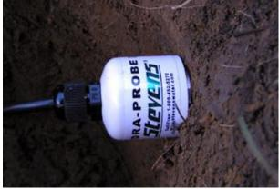
Figure 2.6 HydraProbe Installed in undisturbed soil.
